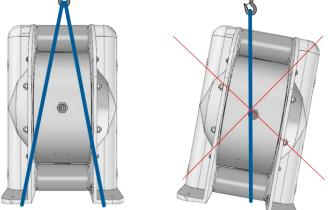
Never lift the pump under pressure.
