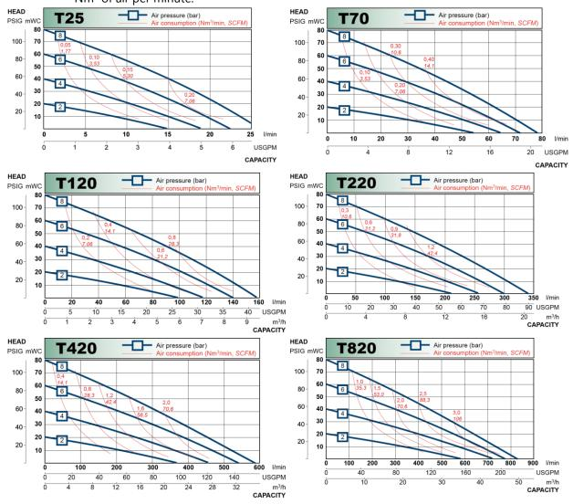
Recommended flow is half of the max flow, e.g. recommended flow for a T70 is 35 l/min.
