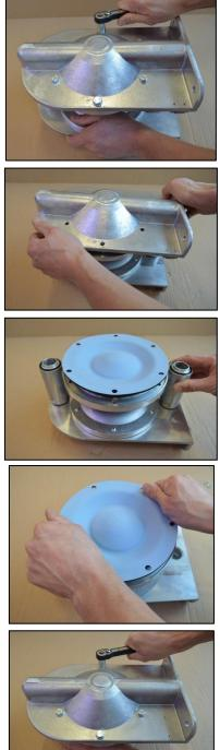
Fig. 3.5.1 Unscrew the housing screws [37] on one side of the pump.
